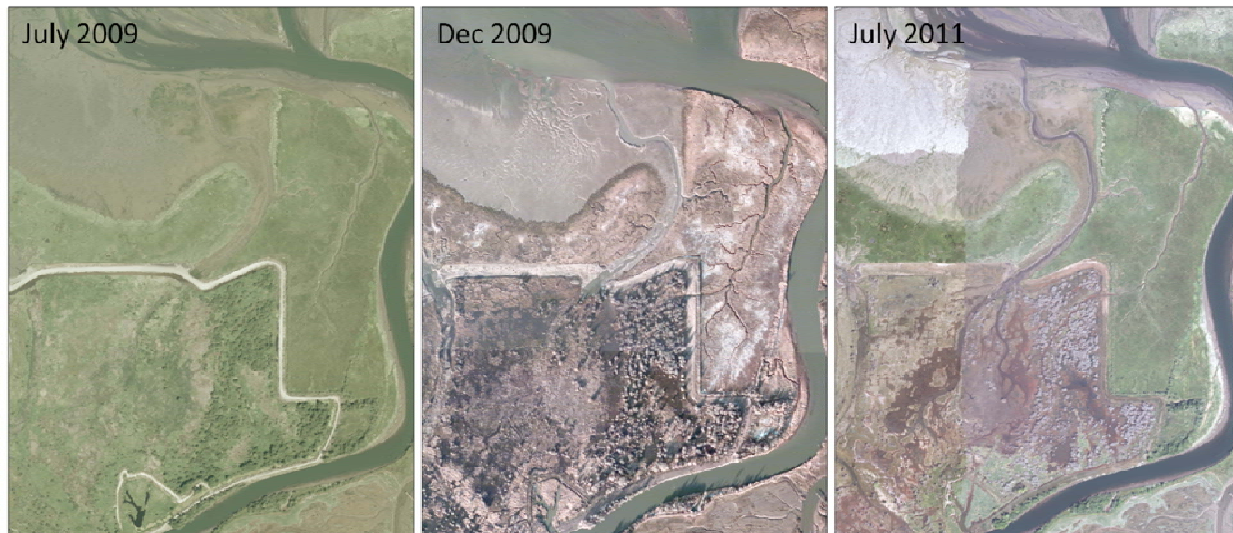
FIGURE 12. TRUE COLOR AERIAL PHOTOGRAPHS SHOWING CHANNEL DEVELOPMENT AT RESTORED UNIT 3 TIDAL CHANNEL.
